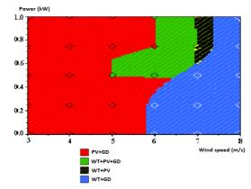
Fig. 2. Produced power from various system resources to feed the network in desert areas in Algeria.
