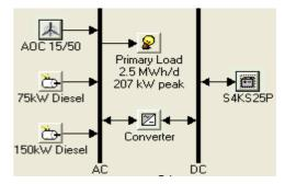
Fig. 4. The electrical installation to be studied on HOMER.
