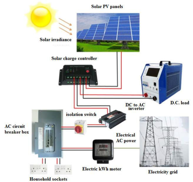
Fig. 3. Components of an on-grid PV system.
