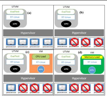
Fig. 6. (a) Scenario 1: One-to-All (b) Scenario 2: One-to-One (affinity) in Hyper-V (c) Scenario 3: Contention with 1 CPU-Load VM atop Hyper-V (d) Scenario 4: Contention with one Memory-Load VM atop Hyper-V
