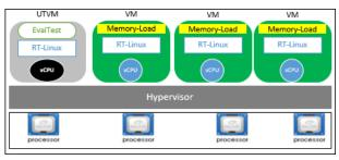
Fig. 8. Scenario 6: All-to-All with three memory-Load VMs
