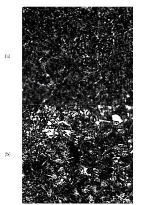
Fig. 4. Micrograph after carburizing at  $900C^{\circ}$  and quenching for 3h. (a) Surface zone, (b) inner area.
