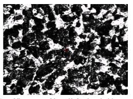
Fig. 1. Microstructure of the steel before the carburizing treatment.
