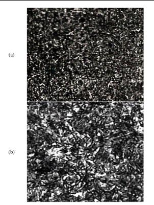
Fig. 3. Micrograph after carburizing at  $900C^{\circ}$  and quenching for 2h. (a) Surface zone,(b) inner area.
