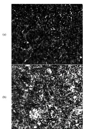
Fig. 2. Micrograph after carburizing at  $900C^{\circ}$  and quenching for 1h. (a) Surface zone,(b) inner area.
