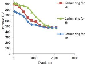
Fig. 8. Hardness of steel carburized at 900°C for 1, 2, and 3 hours.
