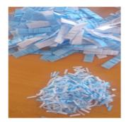
Fig. 2. Shredded single-use surgical face masks.
