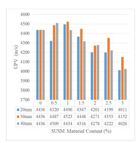
Fig. 9. UPV of concrete with different contents and lengths of SUSFM fibers.
