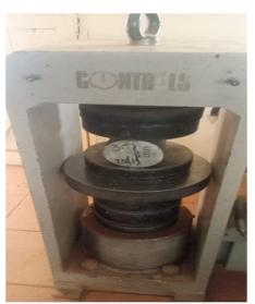
Fig. 5. Concrete split tensile strength testing.
