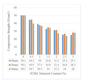
Fig. 7. Compressive strength of concrete with different contents and lengths of SUSFM fibers.
