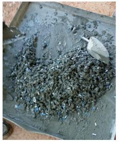
Fig. 3. Mixing of concrete with added SUSFM fibers.
