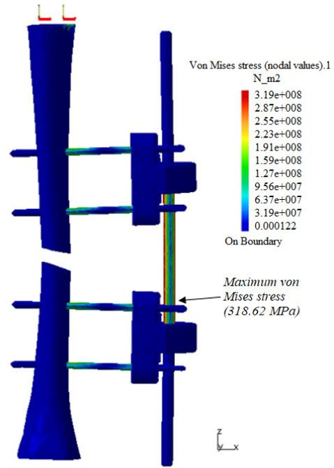
Fig. 6. Von Mises stress distribution.
