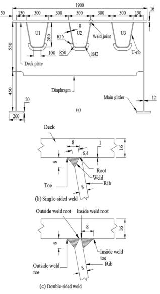
Fig. 5. Dimensional details of (a) the cross-section of the full-span bridge, (b) single-sided weld, and (c) double-sided weld.
