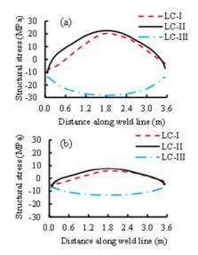
Fig. 9. Stress histogram of double-sided weld at joint 1: (a) Outer weld toe, and (b) outer weld root.
