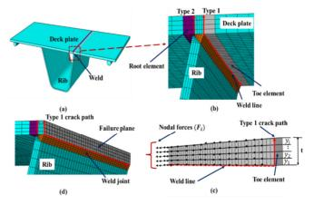
Fig. 2. The 3D solid element model in structural stress calculation.
