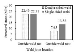
Fig. 10. Comparison of structural stress of weld joints under LC-II.
