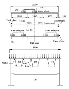
Fig. 7. Loading conditions: (a) longitudinal load positions and (b) constant transverse loading (in mm).
