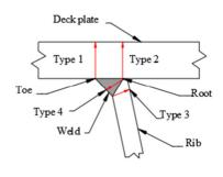
Fig. 1. Rib-deck weld joints.
