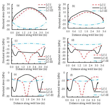
Fig. 8. Stress histogram of single-sided weld joints: (a) Outside weld toe at joint 1, (b) outside weld root at joint 1. (c) outside weld toe at joint 2, (d) outside weld root at joint 2, (e) outside weld toe at joint 3, and (f) outside weld root at joint 3 for different loading positions.
