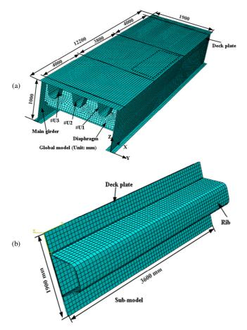
Fig. 6. FE simulation of (a) global shell-model and (b) solid sub-model.
