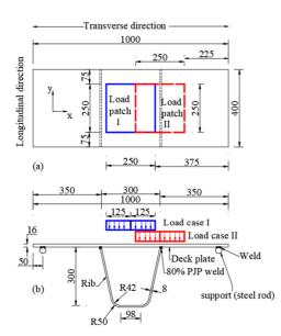
Fig. 3. Dimensional details and loading condition of the model.
