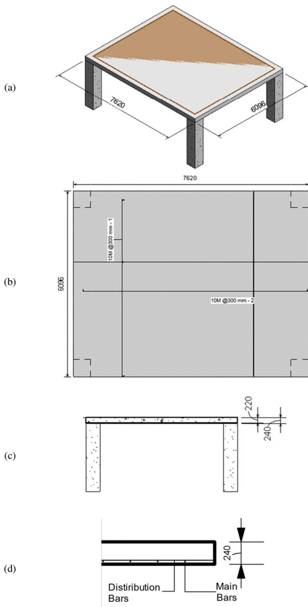
Fig. 1. Flat plate system details: (a) 3D view, (b) top view, (c) longitudinal section, (d) cross section.
