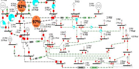
Fig. 7. UPFC located in line 2–6 (line 4-6 is shown in red despite 97% capacity).
