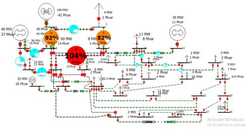
Fig. 5. System overload on line 4-6 of a modified IEEE 30 bus.
