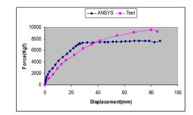
Fig. 5. Force-displacement curve obtained from finite element analysis for sample 3
