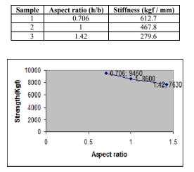
Fig. 7. Relationship between ultimate strength of the steel shear wall and aspect ratio of the panel
