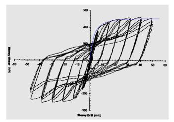
Fig. 2. Comparison of the finite element results (blue ANSYS) and the sample tested under cyclic load (Black)
