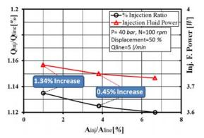
Fig. 5. Effect of the size of the pipeline on the injection capacity and the injection fluid power at 50% VDRIP displacement.
