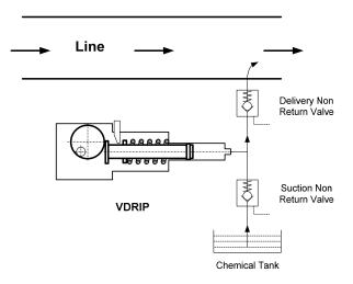
Fig. 11. Schematic diagram of the VDRIP principal.
