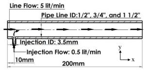
Fig. 6. Schematic diagram of the 3D-CDF test-section
