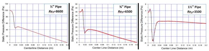
Fig. 8. Effect of cross flow injection on the line pressure difference distribution along x-axis, 3D-CFD ANSYS Fluent analyses
