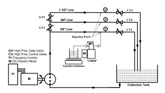
Fig. 1. Schematic diagram of the test-rig.
