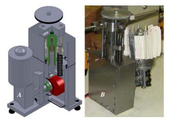
Fig. 12. A:3D-CAD of the VDRIP, B: Photograph of the realized VDRIP.
