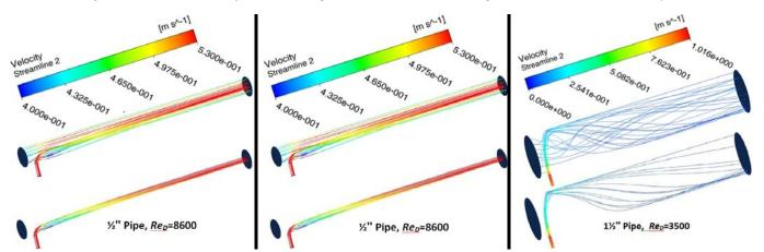
Fig. 9. Stream lines including cross flow injection, 3D-CFD ANSYS Fluent analyses
