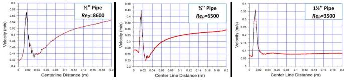
Fig. 7. Effect of cross flow injection on the line velocity magnitude along x-axis, 3D-CFD ANSYS Fluent analyses
