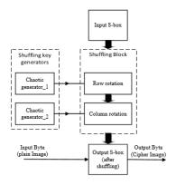
Fig. 2. Block diagram of proposed algorithm
