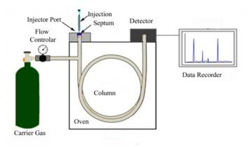
Fig. 1. A typical schematic diagram of a gas chromatograph with a thermal conductivity detector.
