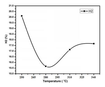
Fig. 6. Variation of hydrogen percentage of the evolved gases with increasing temperature
