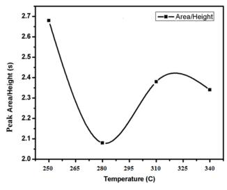
Fig. 8. Peak area/height ratio with increasing reactor temperature.
