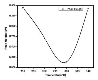
Fig. 7. Variation of peak height with the temperature of the evolved gases
