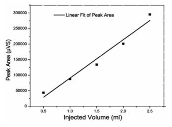
Fig. 3. Linear fit of the peak area versus volume of pure hydrogen
