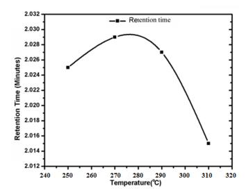
Fig. 5. Retention time of evolved hydrogen versus temperature of reactor
