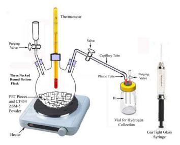
Fig. 2. A schematic diagram of experimental arrangements of the reactor for hydrogen production and collection
