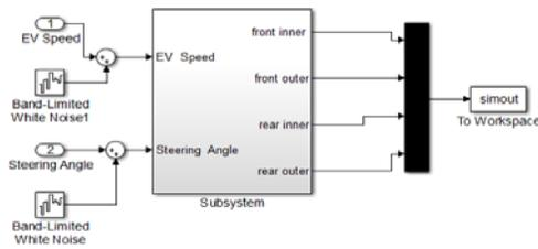
Fig. 3. Matlab/Simulink model of EDS.
