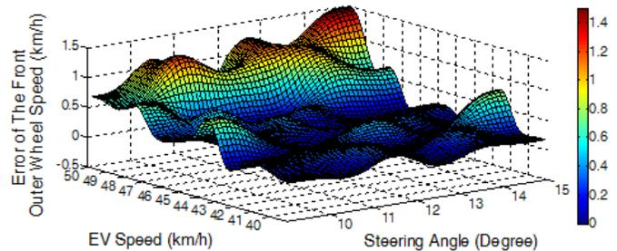
Fig. 11. Difference between Simulink and RBNN results of front outer wheel.
