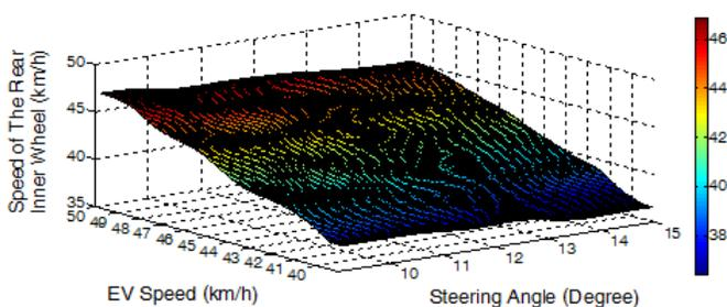
Fig. 8. RBNN results of rear inner wheel (40 dB).
