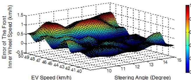
Fig. 10. Difference between Simulink and RBNN results of front inner wheel.
