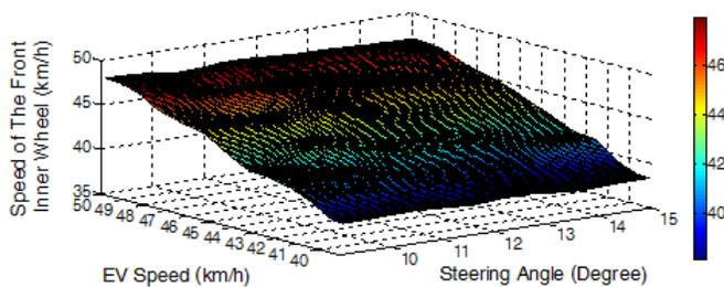
Fig. 6. RBNN results of front inner wheel (40 dB).
