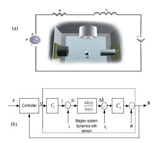
Fig. 1. (a) Electrical Circuit Model of Maglev System (b) Schematic Block Diagram of Maglev System.
