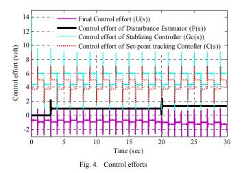
From Figure 4, it is clearly noticed that the designed control scheme has ability to track the desired set-point input reference trajectory and remove the effect of external disturbances. The disturbance estimator works only when the system is subjected to external disturbances, as clearly seen at time 3 second and 20 second. The overall control effort is
