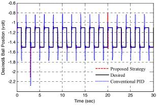
Fig. 5. Desired & Ball Position (Comparative)
