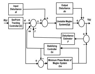
Fig. 2. Block diagram of 2-DOF control strategy
