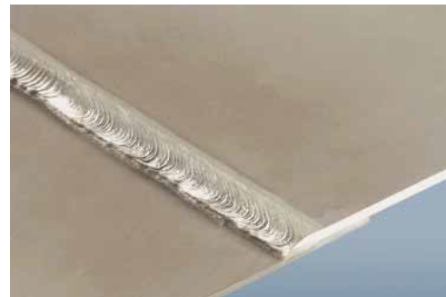
Fig.6. Overlapped welding made with the CMT process between an upper aluminium sheet and a lower steel sheet. Source: Fronius
