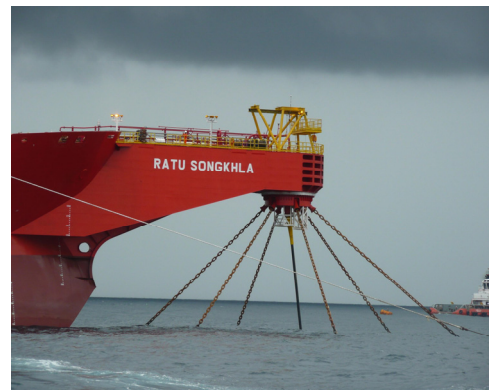
Photo 7. Modified hull with turret
