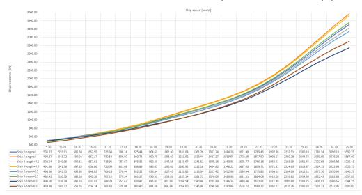
Fig.10. Ships resistance for the initial Ship 2, Ship 5 and for new derivated 6 ship hulls
