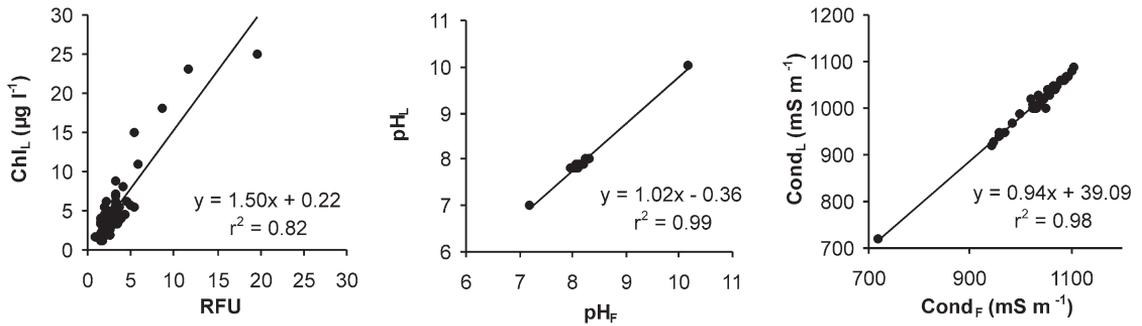
Fig. 4. The correspondence between the field measurements and laboratory results of chlorophyll-a, pH and conductivity.
