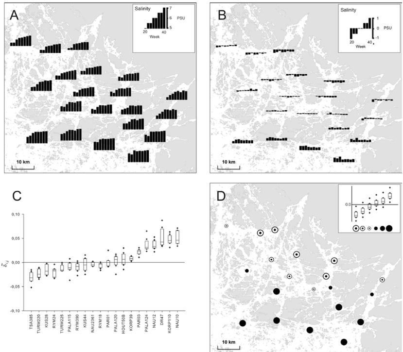
Fig. 8. Salinity in May-October in 2007. A) Surface-layer salinity, B) Salinity deviations from the median of the corresponding week, C) Time stability plot, indicating station-wise stability of the relative deviations from the global median of the corresponding week, D) Classification of the stations according to the location of the median, and 25<sup>th</sup> and 75<sup>th</sup> quartiles.
