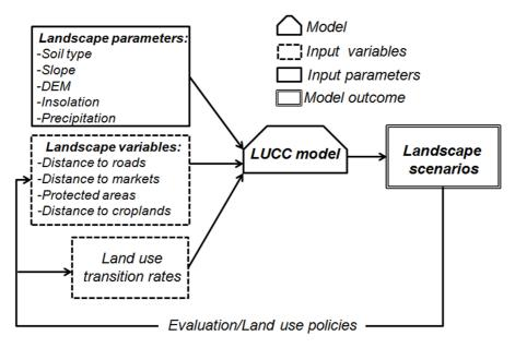
Fig. 3. General description of the modeling framework, in which landscape attributes obtained using remote sensing and GIS techniques are used as inputs for a LUCC model. The model evaluates the role of each attribute in the land changes and simulates future landscape scenarios (adapted from Maeda et al. 2011a).
