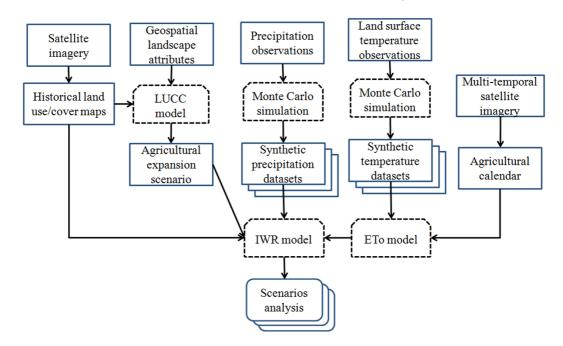
Fig. 5. Flow chart illustrating the integrated modelling framework concept used in assessing the potential impacts of agricultural expansion and climate change on irrigation water requirements (adapted from Maeda et al. 2011b).
