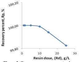
Figure 2. Copper recovery percent using a regeneration solution of 2eq HCl/L and varying dried exhausted resin dose
