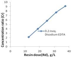
Figure 5. Copper concentration ratio using a regeneration solution of disodium EDTA and varying dried exhausted resin dose
