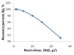
Figure 4. Copper recovery percent using a regeneration solution of 2eq H<sub>2</sub>SO<sub>4</sub>/L and varying dried exhausted resin dose
