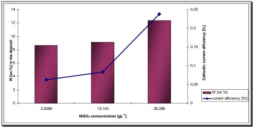
Figure 2. Effect of NiSO<sub>4</sub> concentration on the CE% and on W% of Ni–W alloy codeposited from NiW solution (I=1 A, pH = 8, t = 30 min.,  $25 ^{\circ}\text{C}$ ).
