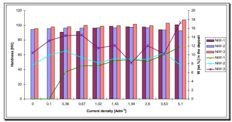
Figure 5. The influence of current density on hardness and the W content in the deposit of NiW alloy
