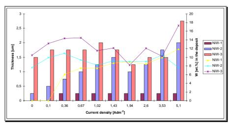
Figure 4. The influence of current density on thickness and the W content in the deposit of NiW alloy
