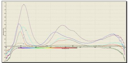
**Figure 1.** Overlapping spectra of UV - VIS - NIR range for the following solutions:  $1-131.944~g \cdot L^{-1}~Na_2WO_4 \cdot 2H_2O$ ,  $2-131.944~g \cdot L^{-1}~Na_2WO_4 \cdot 2H_2O + 147~g \cdot L^{-1}~C_2H_5Na_3O_7 \cdot 2H_2O$ , 3-NiW-1~bath,  $4-26.286~g \cdot L^{-1}~NiSO_4 \cdot 6H_2O$ ,  $5-26.286~g \cdot L^{-1}~NiSO_4 \cdot 6H_2O + 147~g \cdot L^{-1}~C_2H_5Na_3O_7 \cdot 2H_2O$ , 6-NiW-2~bath, 7-NiW-3~bath
