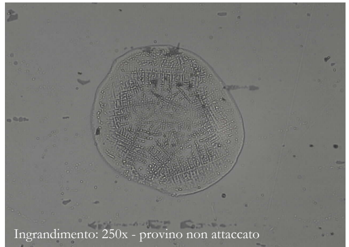
Figura 29: Struttura dendritica provino centrale attacco D. Figure 29: Attachment D, central specimen dendritic structure.
