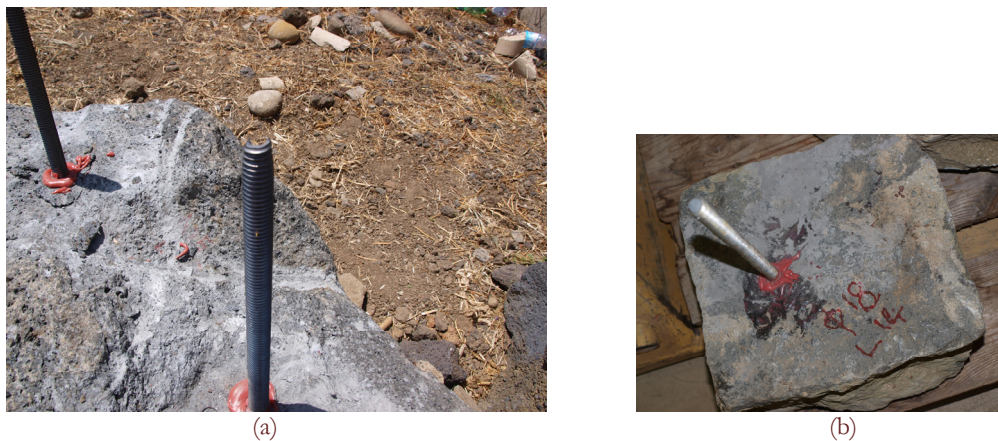
Figure 2: Typical failure mechanisms in the case L=10\phi . Basalt test B-10-10-1 (a) and limestone test C-14-10-2 (b).
