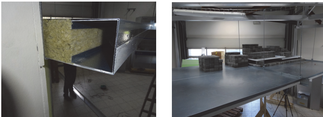
Figure 1: Detail of panel of suspended ceiling (left) suspended ceiling with surface load and 6x point load (right).
