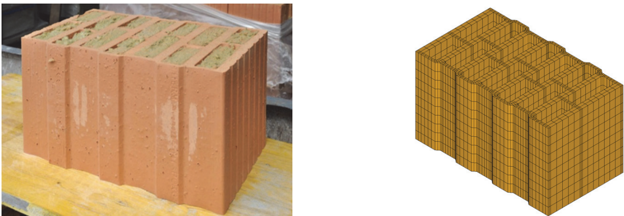
Figure 1: Masonry block used in experimental walls and FEM model of masonry block.
