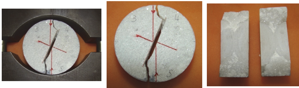
Figure 12: A typical CCNBD specimen fractured under mode II loading.
