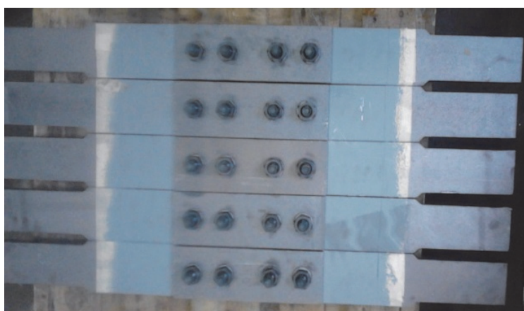
Figure 11: Blasted and half-coated specimens.
