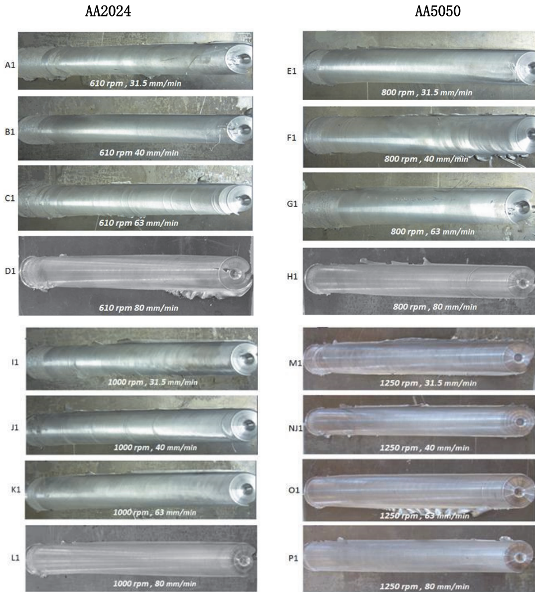
Figure 7: Welded specimens in different rotation and forward speeds.
