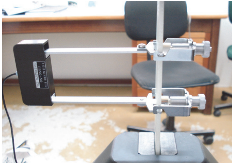
Figure 2: Tensile test set up with an extensometer
