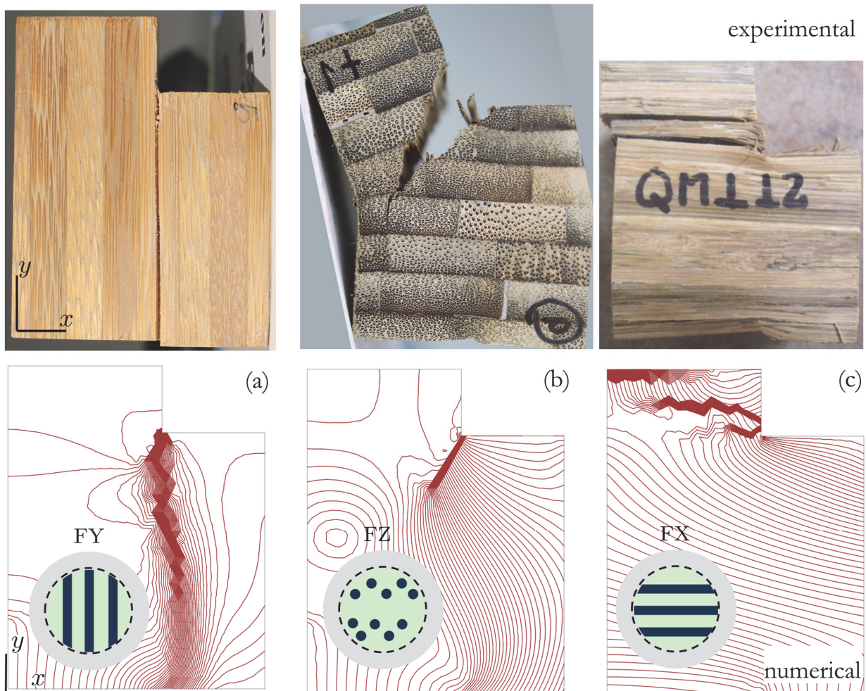
Figure 7: Cracks in the experimental test and the corresponding iso-displacement contour lines in the numerical simulation of LGB specimen subjected to shear stress: (a) FY-fiber direction, (b) FZ-fiber direction and (c) FX-fiber direction.
