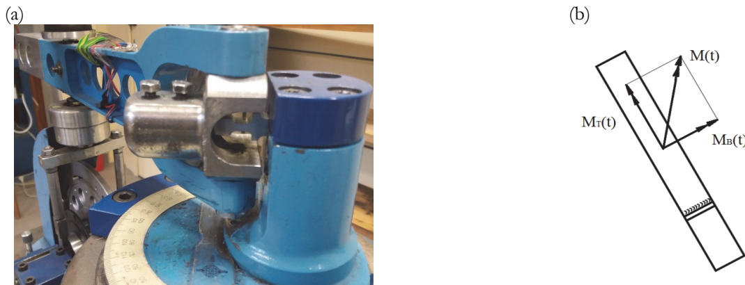
Figure 3: (a) Specimen clamped in MZGS-100 machine, (b) scheme of bending loading applied to the specimen.
