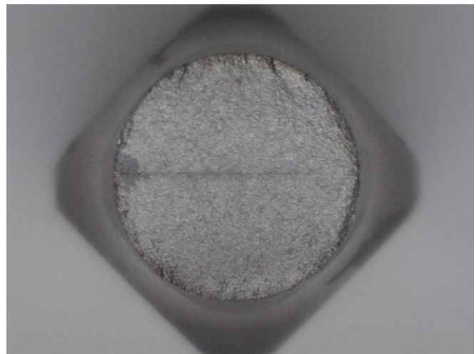
Figure 8: The macroscopic breakthrough of the sample made of steel 16Mo3 after testing under the pendulum bending conditions.
