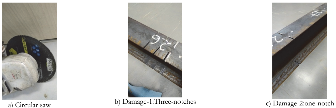
Figure 2: Damage simulations, a) Circular saw, b) Damage-1, c) Damage-2.
