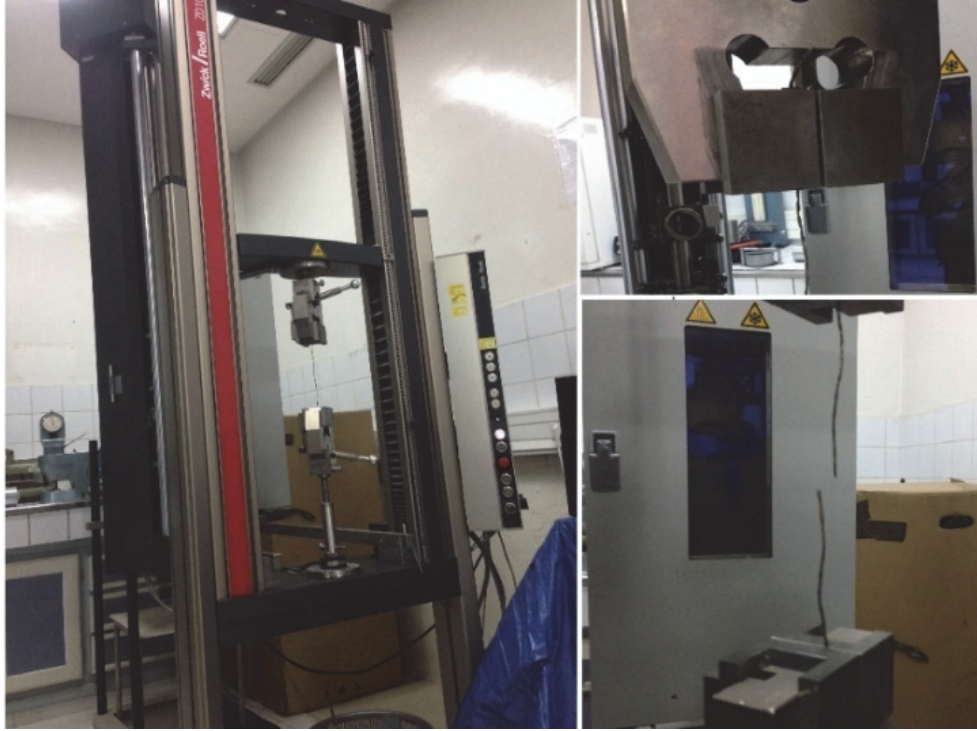
Figure 2. Fitting of test specimens on the testing machine – Zoom on the fixing jaws - Overview of a strand after the tensile test
