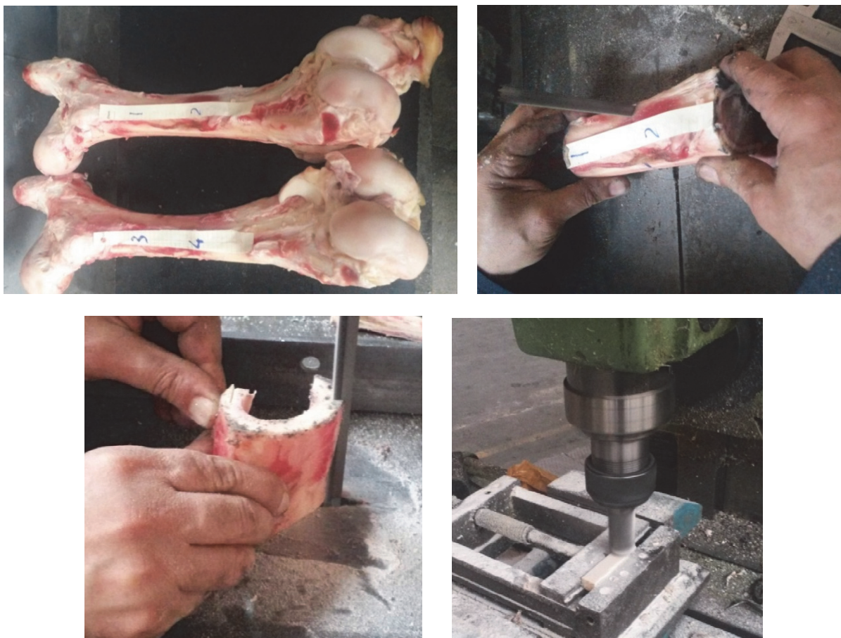
Figure 1: Test specimen preparation from the bovine femur in the shape of rectangular beam samples.
