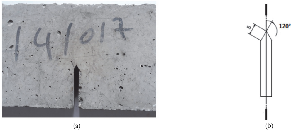
Figure 2: Notch details (a) photo of notched concrete specimen, (b) notch geometry
