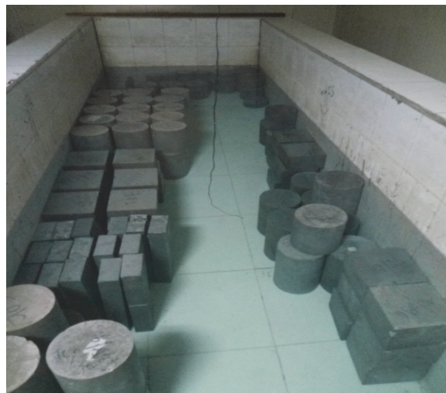
Figure 3: Conservation of concrete specimen in water pool at a temperature of 20^\circ \text{C} \pm 2^\circ \text{C}
