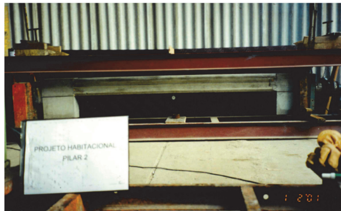
Figure 2: Column positioned for testing.
