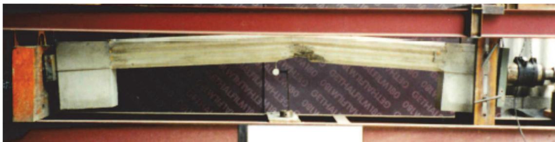
Figure 10: Specimen E1 at the time of rupture in the experimental testing.
