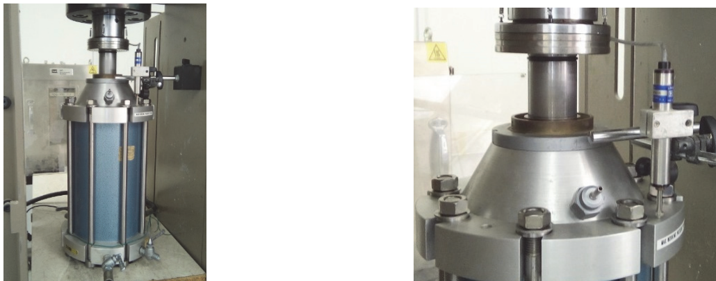
Figure 1: (Left) The triaxial chamber mounted inside the MTS 815 frame; (Right) The external LVDT experimental setup for measuring the axial deformation values during the triaxial compression cyclic tests.
