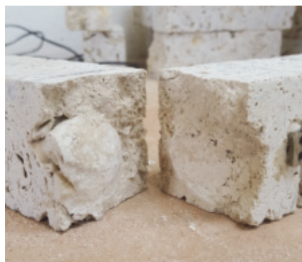
Figure 10: Failure around a mineral build-up (Portland limestone).
