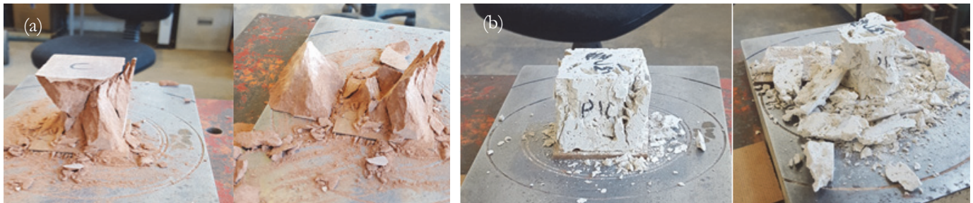
Figure 8: Specimens with uniform failure modes in compression, for (a) Corsehill sandstone and (b) Portland limestone.
