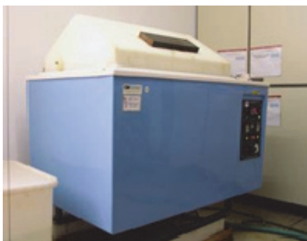
Figure 2: Salt spray fog chamber.
