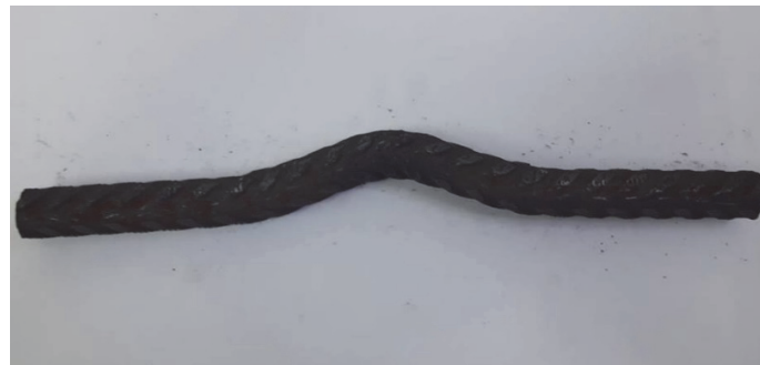
Figure 5: Buckling effect on a tested rebar.
