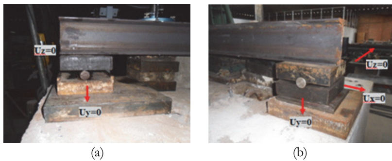
Figure 6: Support conditions of the steel beam specimen [15].
