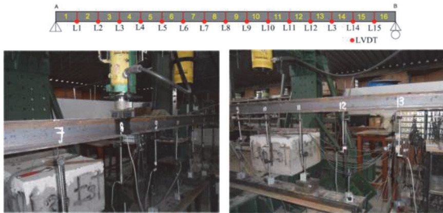
Figure 5: LVDT's positions (16 parts) [15].
