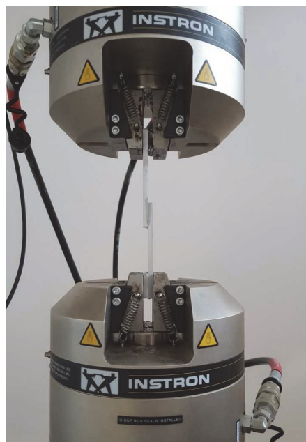
Figure 2: SLJ sample placement at Instron 8801 test machine
