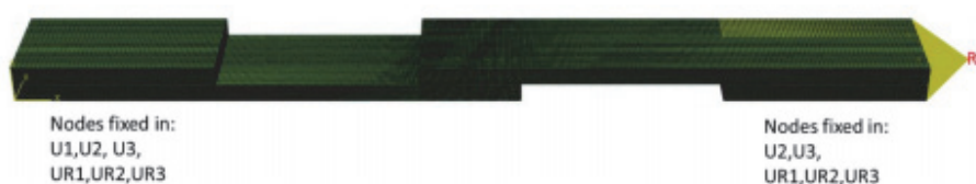
Figure 2: Boundary conditions for the symmetry FE model.
