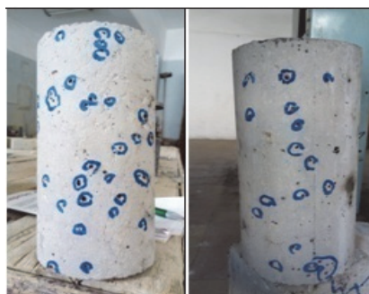
Figure 17: Concrete specimens after exposure to fire
