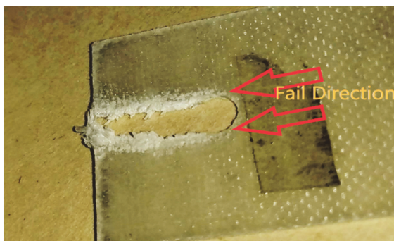
Figure 15: The direction of failure in the specimen under experimental test.
