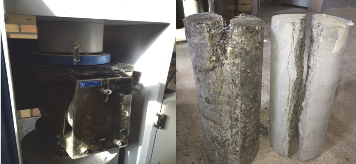
Figure 2: Tensile strength test by the splitting method (left) and failure geometry of specimens (right).
