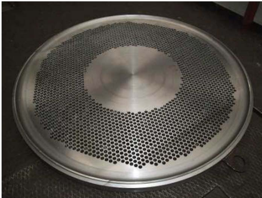
Figure 1: Model of bimetallic perforated plate [3].
