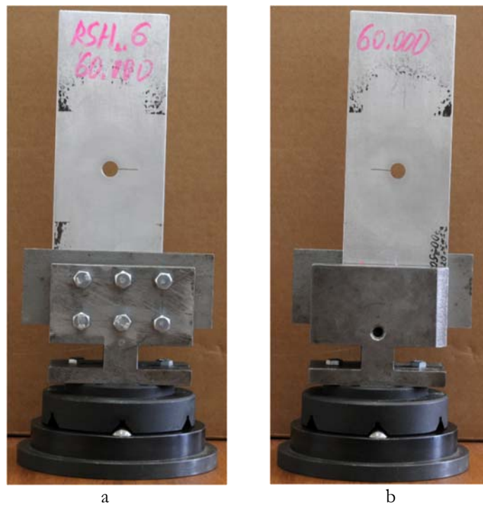
Figure 4: Real view of specimen with non-symmetrical notch clamped in the upper part of kinematically designed mount: measurements on Side A (a) and Side B (b).
