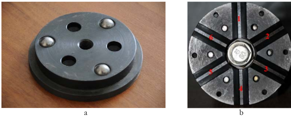
Figure 3: The upper (a) and lower (b) part of kinematically designed mount.
