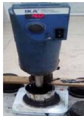
Figure 3: Bitumen modifier apparatus.
